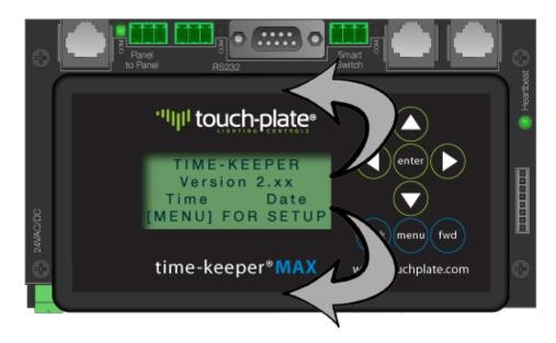
Remove the SD card by pushing it further into the socket until you hear it click and release. You can now remove the SD card. Use a computer to copy the firmware update file TKIII.bin to the SD card and replace the file currently there, or install the new SD card with the firmware file already installed. Install the SD card back into the SD card socket, push it all the way in until you hear it click and release.
