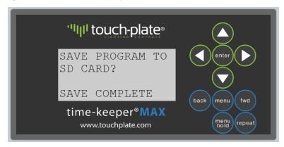
Push the fwd button until you come to the following Update Firmware Screen. Push the enter button to begin the update. A Bootloading Screen will be displayed during the update process.
