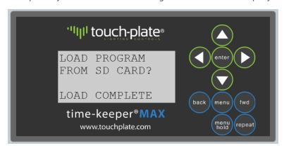
You now need to power cycle the Time-Keeper MAX. When the unit boots to the Main Screen the process is complete. Your Time-Keeper MAX should now be up to date and have all of the original programming loaded onto the unit.
